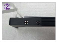
Assembly both below edge of horizon frame and corner with FM3\*4 screw as next photo
