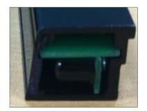
Arrange the frame with black LED on the top and the frame with transparent LED on the bottom between horizon frame 2pcs as top photo
