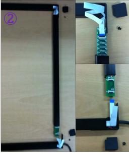
Get the PCB out of the vertical frame as picture and connect the blue FCC with A connector and the white FCC with B connector
