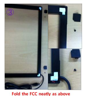
Use FM3\*4 Screws to assemble after arranging FFC the frame with the corner.
